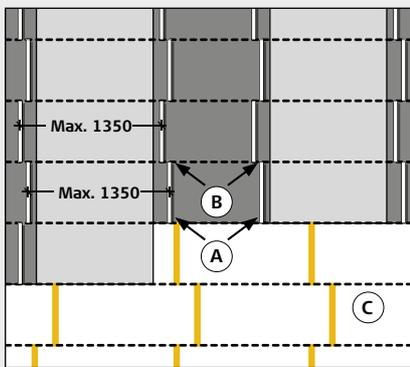
**ABB. 2 PARALLELVERBAND, VERSETZT**
